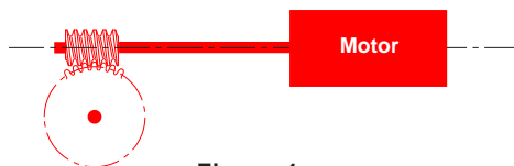
Figure 1 Direct-connected, fixed ratio drive
